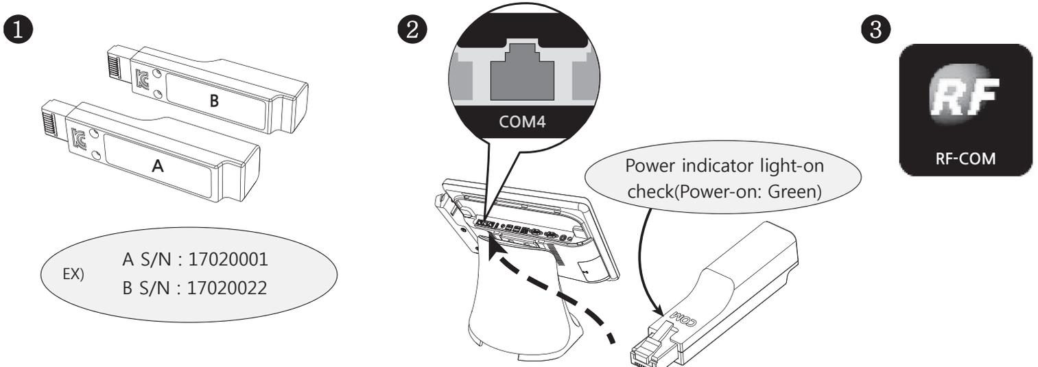
Step 1. Connect "RF-COM A" to P.O.S terminal and run RF-COM program.
